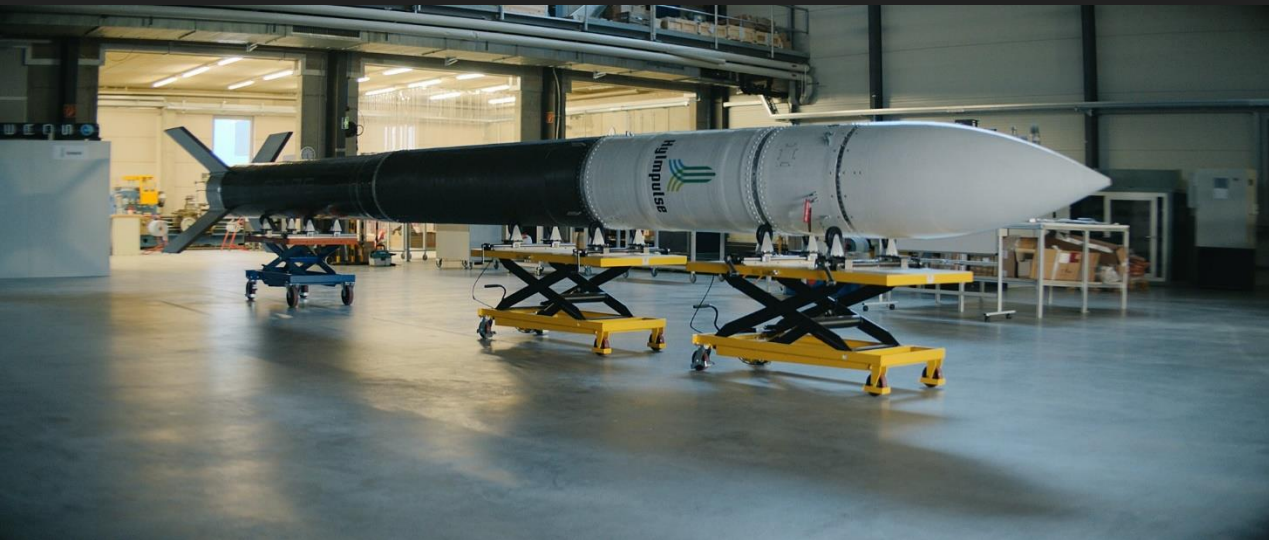
HyImpulse SR75 Test Rocket with 75kN Paraffin Rocket Engine
